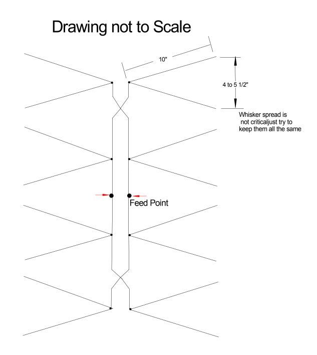
Most any metal will work for the elements. Try to use something near 1/8" diameter and make sure they are free of all coatings and oxidation where they connect to the phase line.
